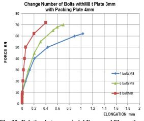
Fig. 32: Relation between Axial Force and Elongation in Case of Change Number Bolts.
