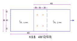
Fig.8: Specimen Geometry
