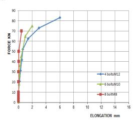
Fig.26: Relation between Axial Force and Elongation in Case of Change Number of Bolts with the Same Area of Bolts.
