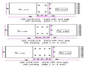
Fig.23: Specimen Geometry in Case of Change Number of Bolts with the Same Area of Bolts.
